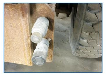
"The ZSi-Foster FF Plus couplers didn't show any white or red rust after a full season of use. They connected and disconnected easily without any leakage."
