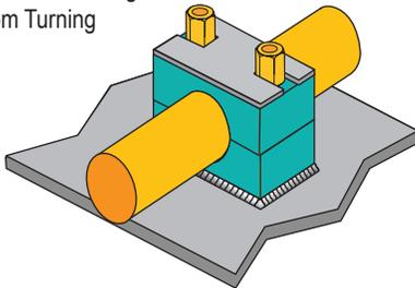
(3) Assemble Another Clamp Onto the Stacking Bolt in Same Manner as Single Clamps are Installed
