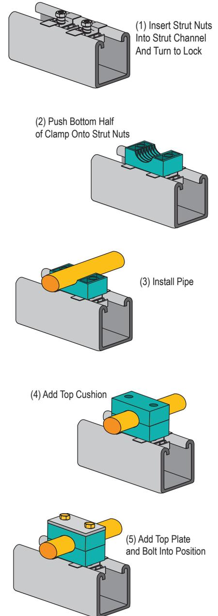
**NOTE:** The ZSA Nut will slide within the Channel so clamp units can be adjusted before being firmly bolted.
