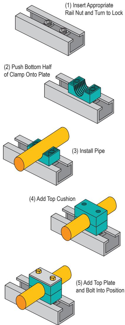
**NOTE:** The rail nut will slide within the rail so clamp units can be adjusted before being firmly bolted.
