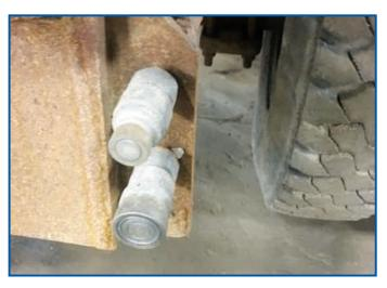
"The ZSi-Foster FF Plus couplers didn't show any white or red rust after a full season of use. They connected and disconnected easily without any leakage."
